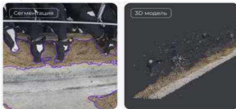
Figure 2 – Computer vision system for monitoring feed intake from the feeding table
