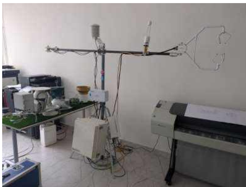
Fig.1 Tower for measuring GHG emission by turbulent pulsation method
